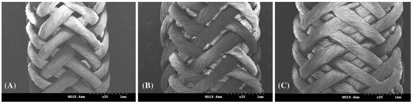
Fig. 3 SEM micrographs of the single- (a), double- (b), and triple-layer (c) microbraided PLA nerve guide conduits
